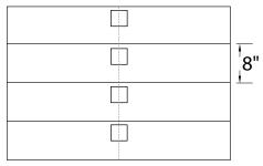
Mount in center of stair as close to the upper tread as possible. For best results use one light per step for steps narrower than 5'.
